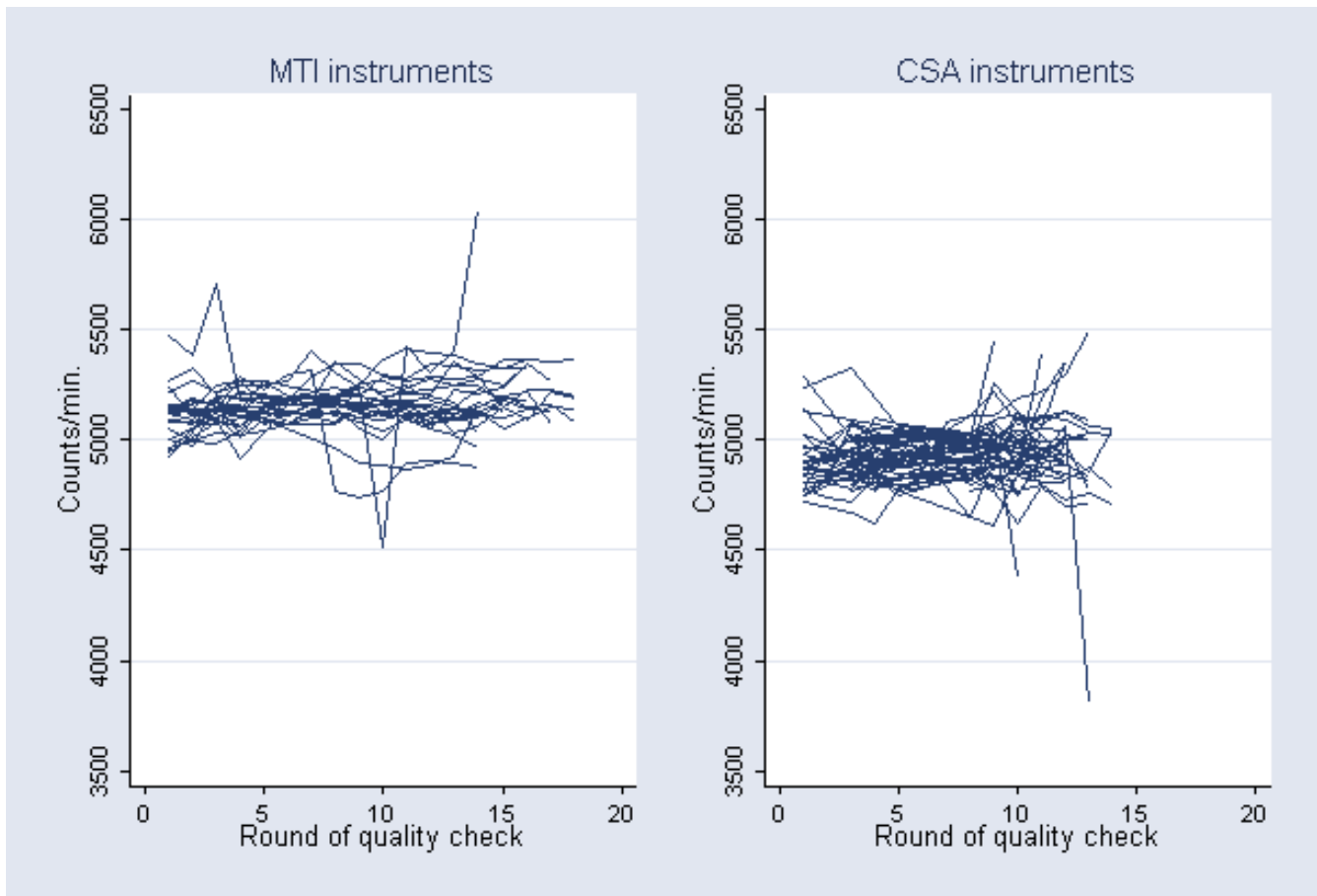
Figure 3 Calibrated instrument output by round of quality check. Within MTI units variation: SD = 110 counts*min -1 . Between MTI units variation: SD = 65 counts*min -1 . Within CSA units variation: SD = 119 counts*min -1 . Between CSA units variation: SD = 67 counts*min -1 .
