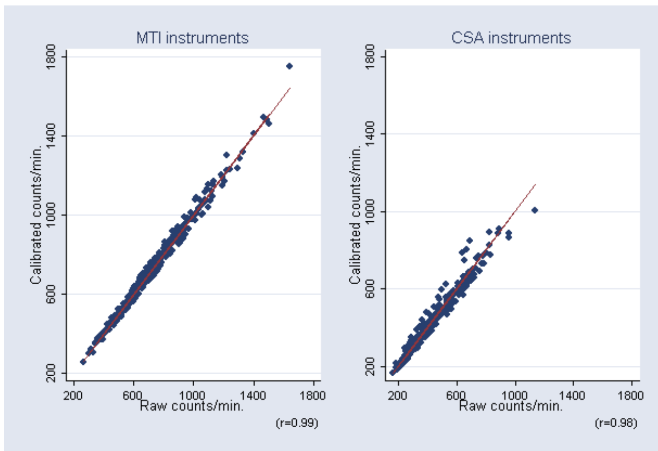
Figure 4 Raw instrument output plotted against calibrated instrument output. Data are obtained in the field.
