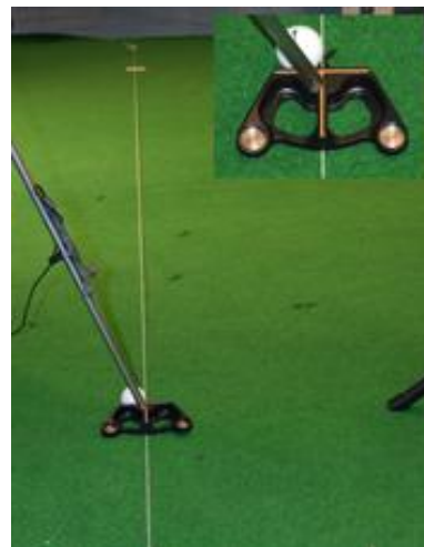
Figure 13. Illustration of how the aim test was done with help of a thread (“3D-method”). This method had a aim variability (expressed as SD ) of 0.19^\circ .
