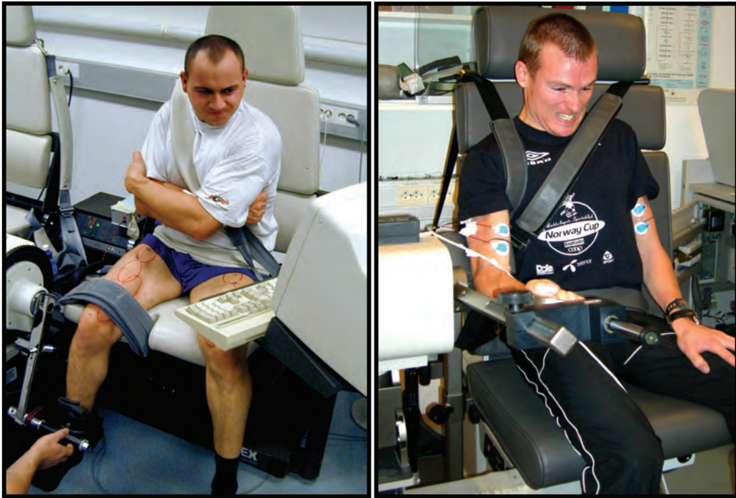
Figure. 3.1. The leg and arm exercises, as well as tests of muscle function before and after exercise, were performed with a dynamometer. In the leg experiment we used a Cybex 6000 (left image), while in the arm experiment we used a Technogym REV 9000 (right image).
