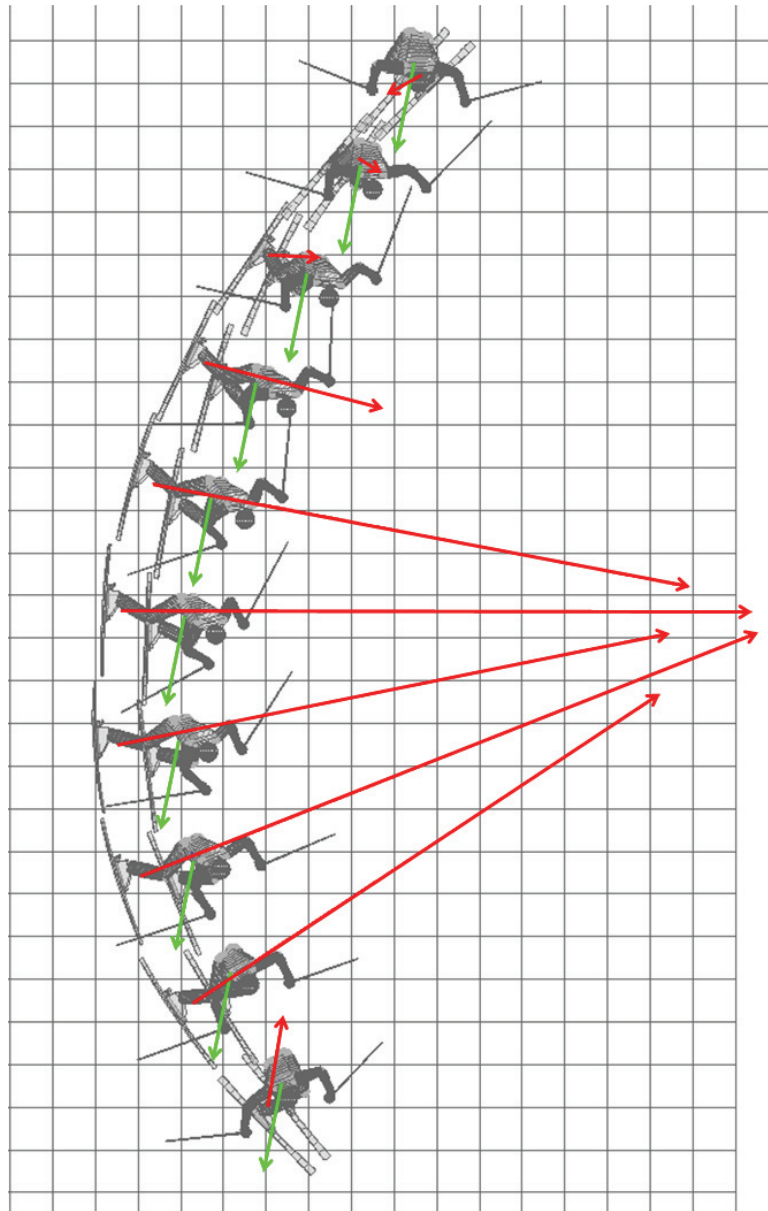
FIGURE 3.14. Free body diagram of a skier from an overhead view showing the changing orientation between the snow reaction force vector (red) and the gravitational force vector (green) over the course of a turn.
