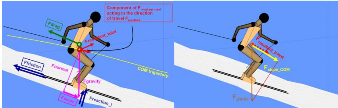
Figure 28: to the left: The external forces acting on the skier and their components in direction of travel. To the right: Definition of F_{slope\_COM} and F_{resultant\_travel} for the force model 1.
