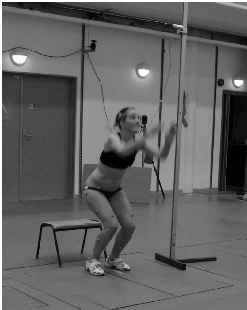
Figure 4.3: The vertical drop-jump. In this project the drop down from box/stool is 30cm, the athletes has placed a foot on each force platform and will try to reach for the overhead target with the head.
