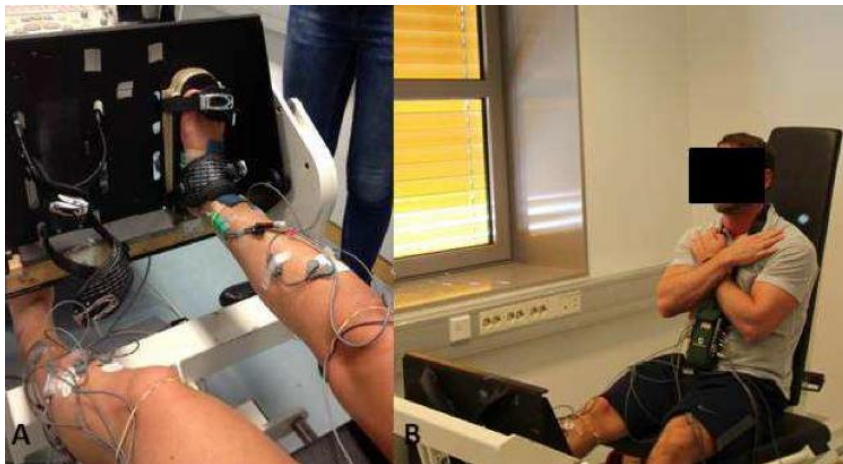
Figure 9: Positioning in the isometric ergometer. A.) Securing of the test foot and positioning of the relaxed foot. B.) General positioning (right) with straight knee, upright back and arms crossed over the chest.
