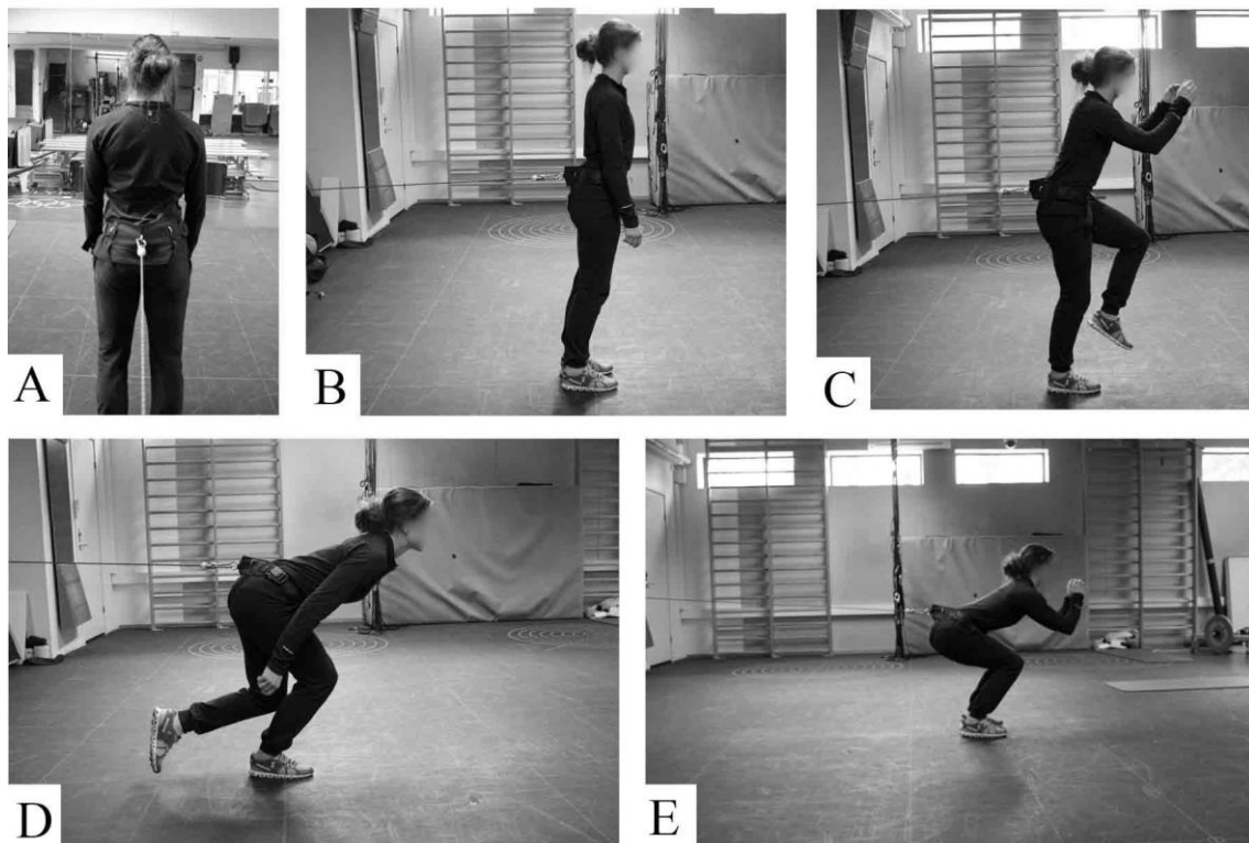
Figure 3.13: Anterior hop test. A) Cable attachment to belt. B) Starting position. C/D) Countermovement phase. D) Start of the concentric phase of the unilateral hop. E) Landing.
