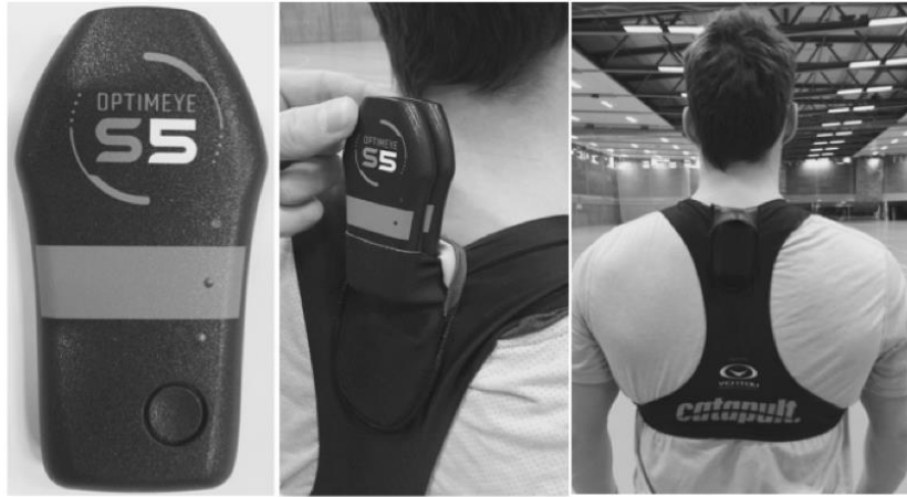
Figure 3.1 The OptimEye S5 device (left). Two devices were taped together (middle), and fitted in a custom-made vest (right) during data collection in a laboratory and field assessment.
