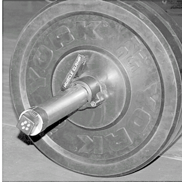
Figure 1. The LED marker and collar assembly placed on the right bar end.
