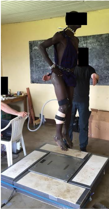
Figure 7: One Maasai subject during flight phase of maximal repetitive jumping. On the bottom of the picture we see the light-weight force plate with the Styrofoam and plywood frame. On the subjects' right leg, we see the strapping of the US probe. Visible on the subjects' right side is also all marker placements.
