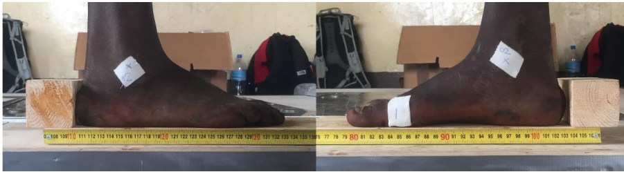
Figure 5: Zoomed-in lateral and medial view of the right foot of one Maasai subject on the custom built measurement board. From these pictures AT moment arm was calculated. Foot length was calculated from medial view pictures with the tip of the toe at center of image. Toe length was calculated from medial view pictures with the hallux at center of image. The images were taken from distance with different centers to minimize distortion.
