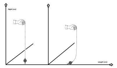
Figure 5: Illustration of the projection of the plumb and the error of measurement that can occur as a consequence of a plumb and the rope.
