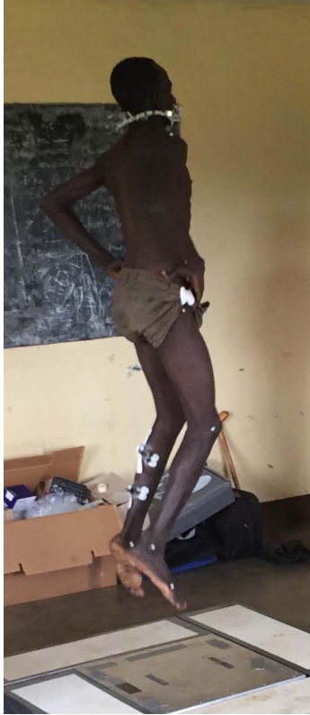
Figure 2: Maasai during the CMJ flight phase. The light-weight force plate including the plywood and Styrofoam frame can be seen in the lower portion of the image. Placement of the reflective markers is visible on the right side of the subject.
