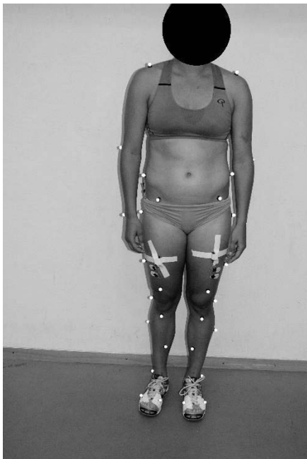
Figure 10: EMG-electrode and reflective marker placement on participant, anterior view
