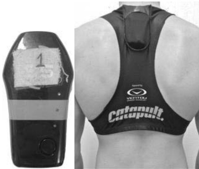
Figure 2.1: The OptimEye S5 (left) fitted in the pouch of a custom-made vest (right). (pictures borrowed from Wik, 2015).
