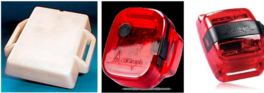
Figure 2: The ActiGraph accelerometers used to assess PA in PANCS1 (model 7164 (left), 4.5 \times 3.5 \times 1 cm, 43g) and PANCS2 (model GT1M (middle), 3.8 \times 3.7 \times 1.8 cm, 27g / GT3X+ (right), 4.6 \times 3.3 \times 1.5 cm, 19g).
