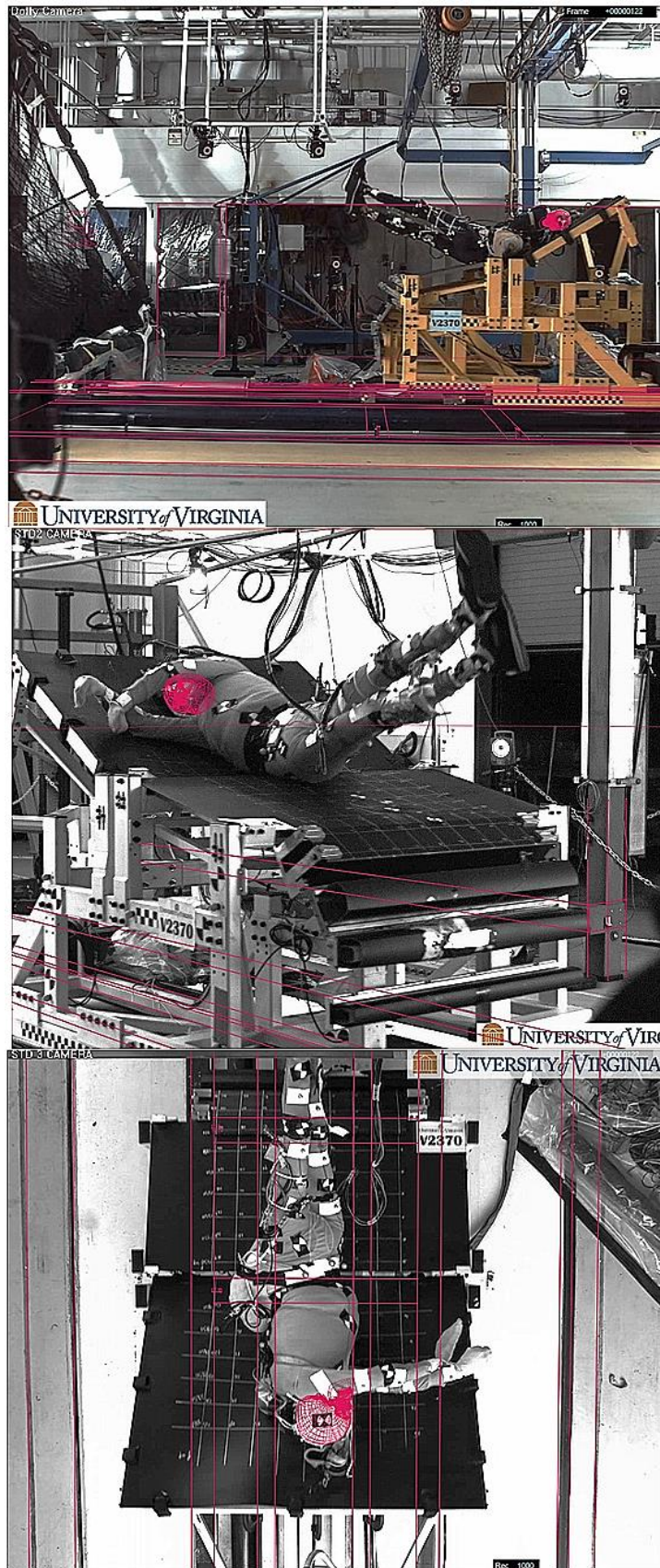
Figure 5: An example of the MBIM skeleton matching with the background video for frame 1 for (a) Camera 1, (b) Camera 2 and (c) Camera 3.
