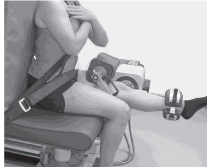
Figure 9. TechnoGym REV 9000 isokinetic dynamometer subject positioning for tests of passive knee extension and contractile function.
