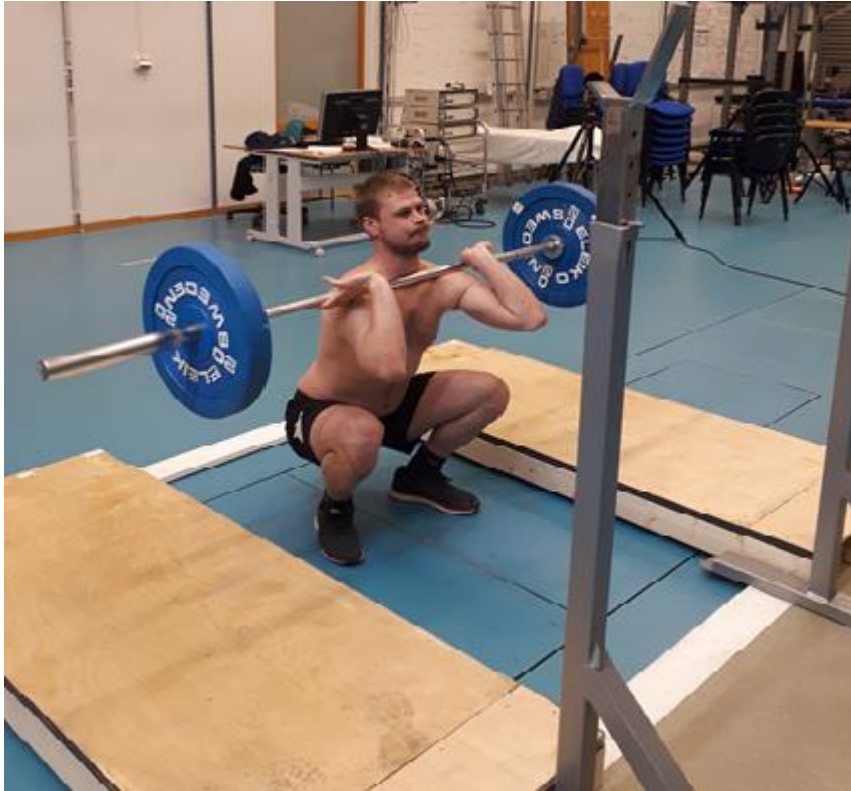
Figure 4: Shows the set- up around the force plates, with the custom made platform and squat stand.
