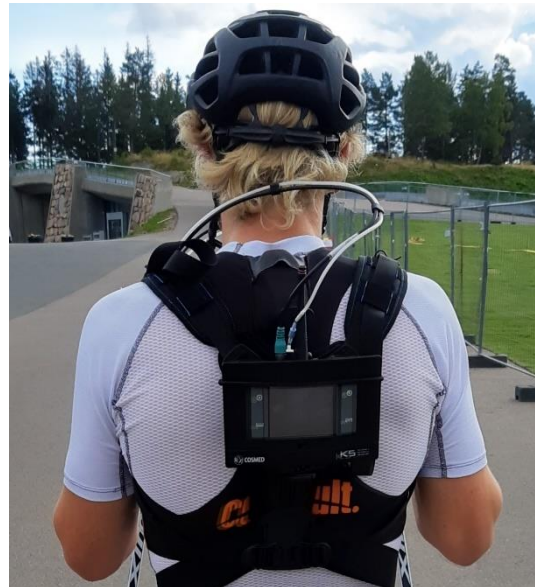
Figure 3: The setup with Cosmed K5 and the upper GPS-unit as used in the field tests.
