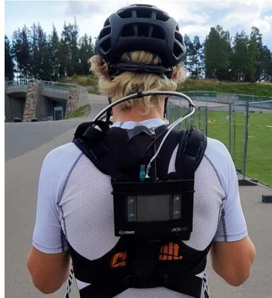
Figure 1.3: The setup with Cosmed K5 and the upper GPS-unit as used in the field tests.
