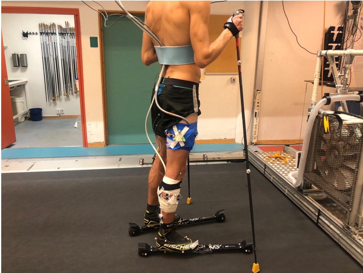
Figure 10. Experimental setup: Participant on the treadmill with ultrasound-transducers, reflective markers, electromyography (EMG) transmitters and force in ski measurement attached. The participant wore an ultrasound-transducer on the gastrocnemius medialis GM and vastus lateralis (VL), however only data from the GM is presented in this study. The cables were held in place by elastic bands around the ankle, knee and abdomen, and ultrasound and force control unit was placed in a box above the participants.
