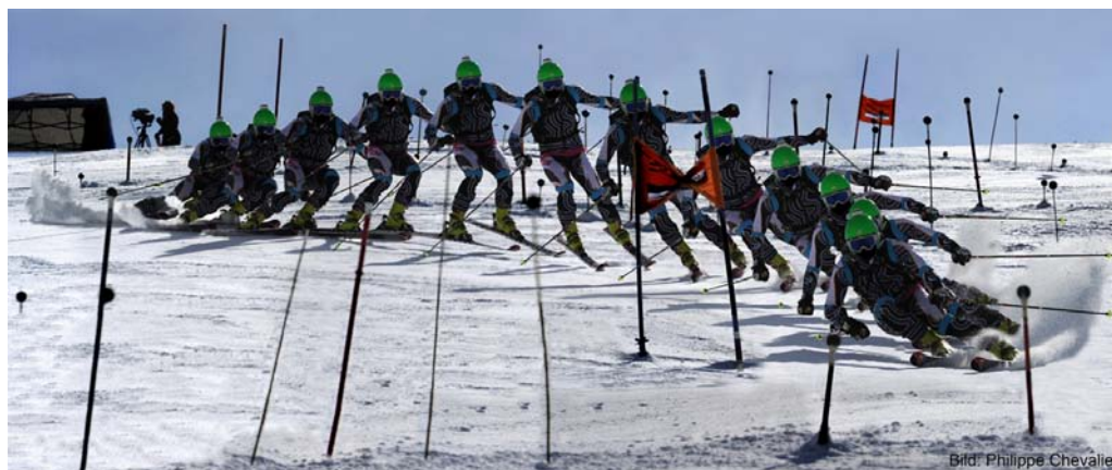
Figure 2. Animation of an alpine skier in the giant slalom course surrounded by the reference points of the reference measurement system at gate number 7 (Photo: Philippe Chevalier).
