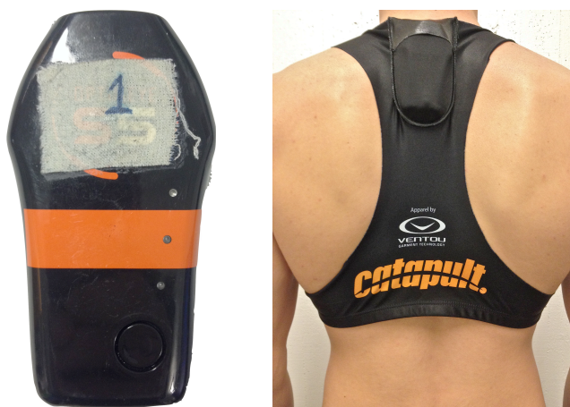
Figure 3 The OptimEye S5 (left) fitted in the pouch of a custom made vest (right).
