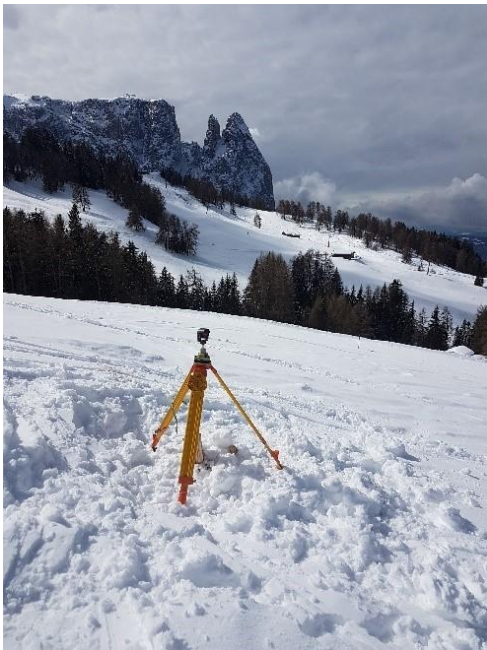
Figure 11: Reference orientation point was measured with differential GNSS/GPS to establish global orientation for QDaedalus system.
