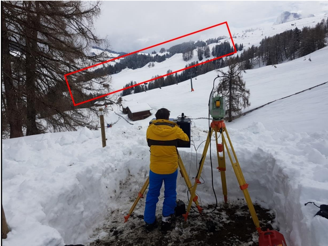
Figure 10: View of the competition course from station 2 of the QDaedalus surveying system position. The red frame highlights the slopestyle course.
