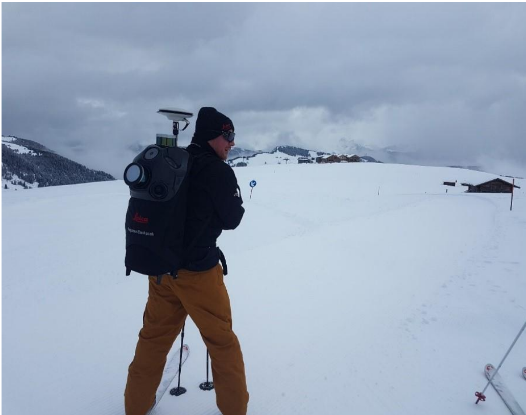
Figure 12: An operator wearing the Leica Pegasus backpack system which was used to establish a point cloud of the snow surface.
