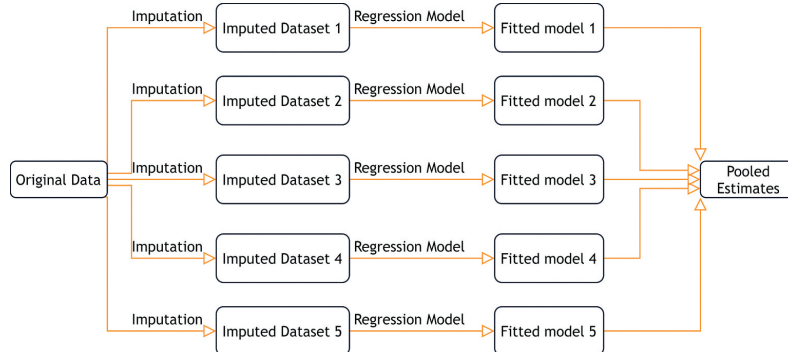
Figure 1. Illustration of the modeling process in the framework of multiple imputation. In the first step, the variables available in the dataset are used to predict m number of potential imputations for the missing observations. A dataset is created for each of the m sets of predictions. The number of imputed datasets, five, is recommended in most cases (Van Buuren 2018, section 2.8). The main model of interest is then run on each of the 5 datasets. The estimates from each model are averaged using Rubin's rules, which calculate standard errors that account for between-imputation variation and the level of uncertainty that stems from the missing data (Sterne et al. 2009; Van Buuren 2018).
