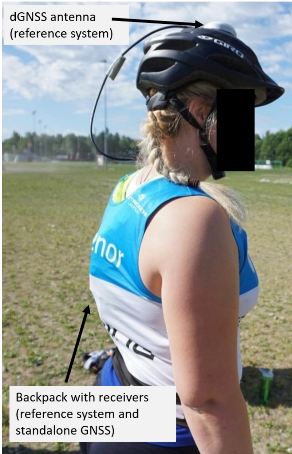
Figure 2 Positioning of the two GNSS systems on participants. The dGNSS reference system antenna was mounted on a helmet and coupled to the receiver in the backpack (hidden under start bib). The standalone GNSS receiver was also placed in the backpack. dGNSS, differential GNSS; GNSS, global navigation satellite system.
