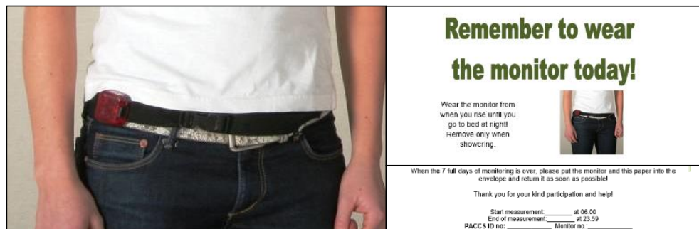
Images 1: The ActiGraph accelerometer used to register physical activity in PACCS (left), together with written instructions for wear (right).
