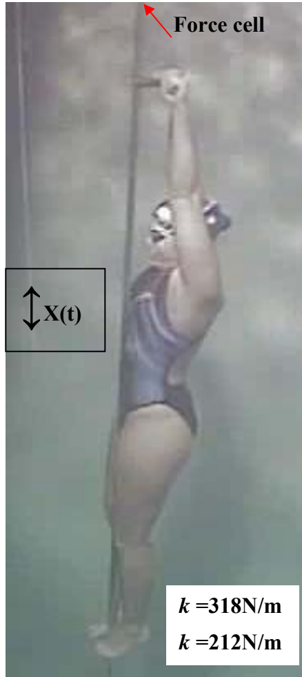
Figure 1: A swimmer attached to the bar during vertical oscillations.
