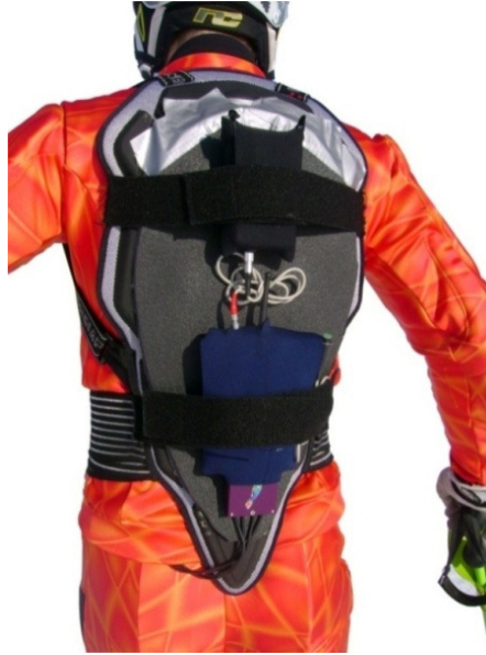
Figure 4.2: An athlete carrying the Pedar system; data log, battery and cables inside the ski pants.
