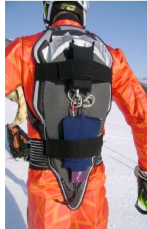
Figure 1. Data logging was accomplished with a portable acquisition system carried in a small backpack. Cables to the insole system were routed underneath a skier's standard suit.
