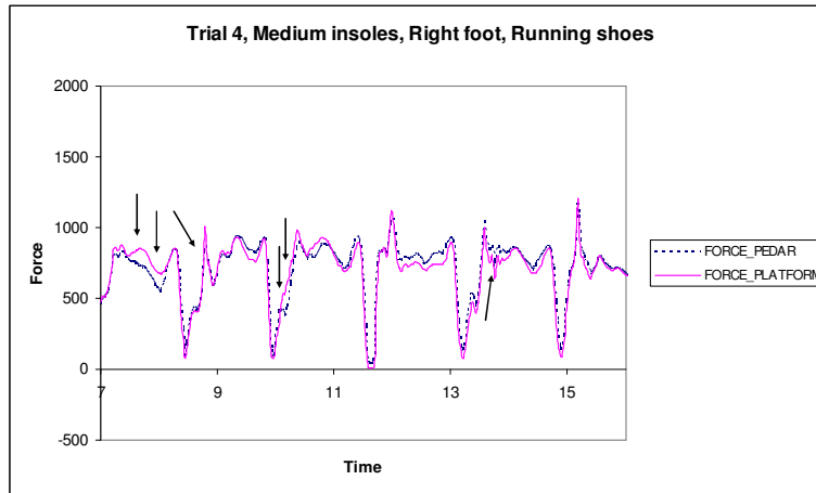
Figure 1. Force-time curves for Pedar and force platform measurements of a subject wearing running shoes. Arrows indicate largest sources of error.
