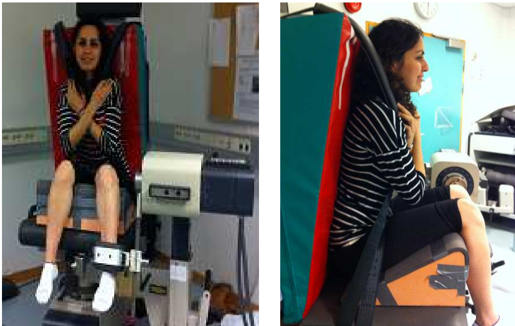
Fig. 2.2. Position of subject on an isokinetic dynamometer (Techno gym Rev 9000)
