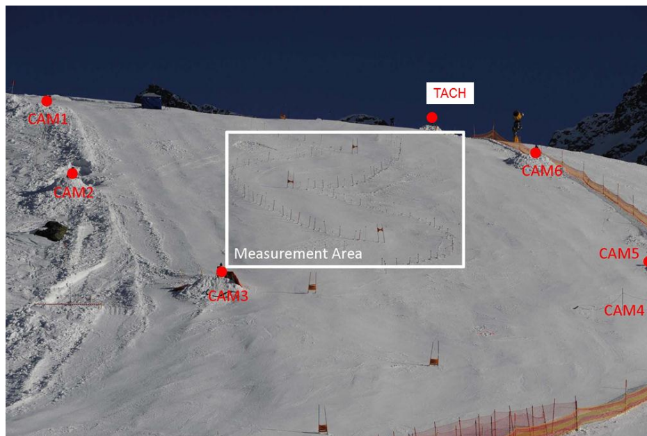
Figure 4. Location of the experimental setup of the validation studies paper I and II. Video camera locations are indicated with “CAM”. The tachymeter location is marked with “TACH”. The area covered by the video based 3D kinematics was accomplished is marked with a white frame. Photo: Philippe Chevalier.
