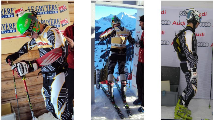
Figure 8. Forerunner equipped with a GNSS receiver in a cushioned camelbag. The receiver is connected with a cable to a GNSS antenna mounted on the helmet.
