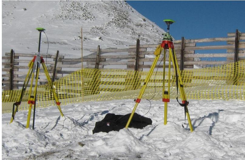
Figure 9. Two GNSS base stations mounted at the start of the downhill race in Lake Louise. Antennas in green mounted on tripods, the receivers and batteries protected in black boxes.
