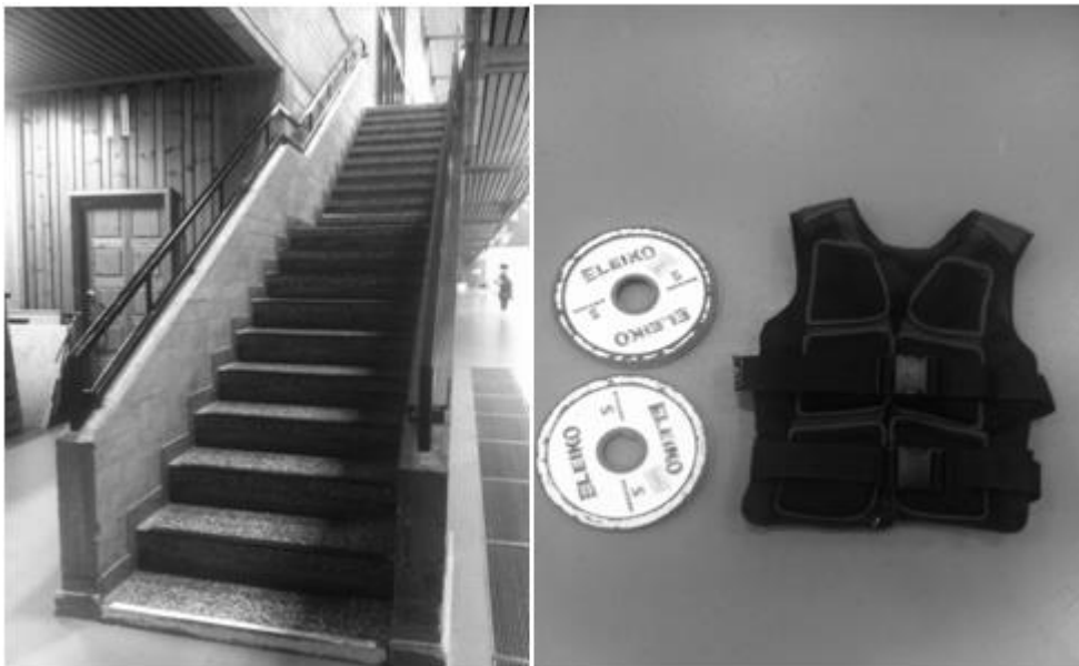
Figure 3.7: The stair and added weights (10.1 kg vest and two 5 kg weight discs) used for the Timed stair climb trials.
