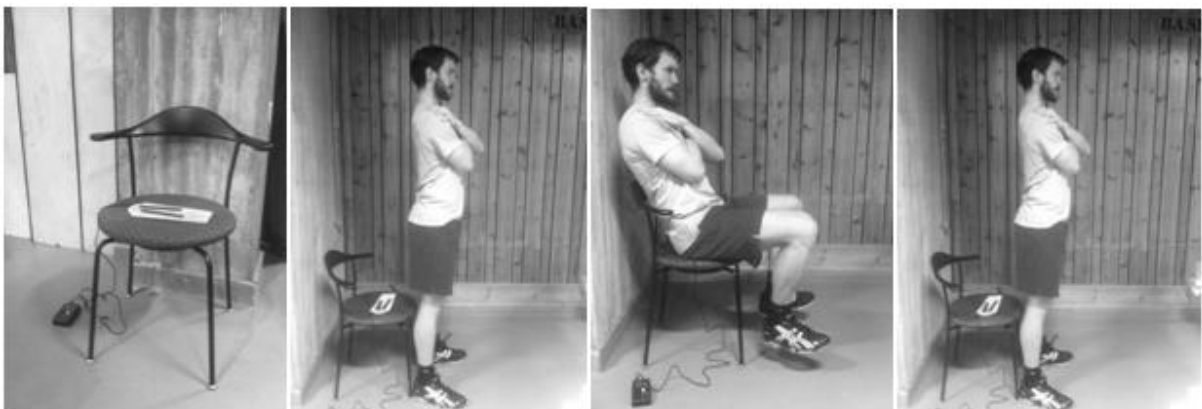
Figure 3.8: illustration of both the equipment used (left) and satisfactory execution of the protocol for the sit-to stand test.
