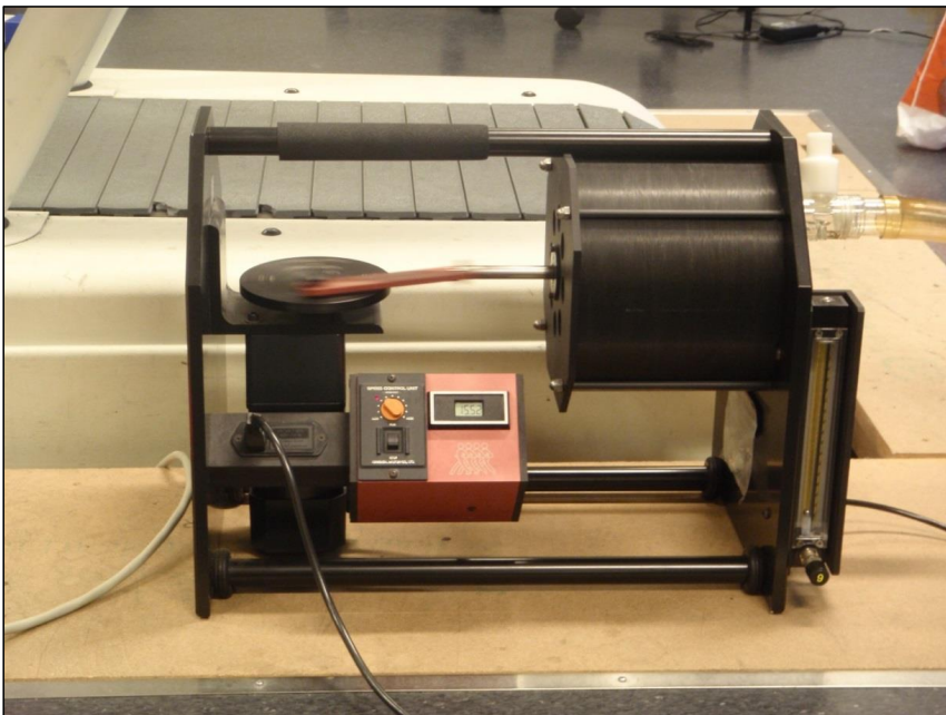
Figure 10. Checking the precision and accuracy of the metabolic equipment at the University of Agder, Kristiansand, using a motorized mechanical lung (VacuMed, Ventura, USA).
