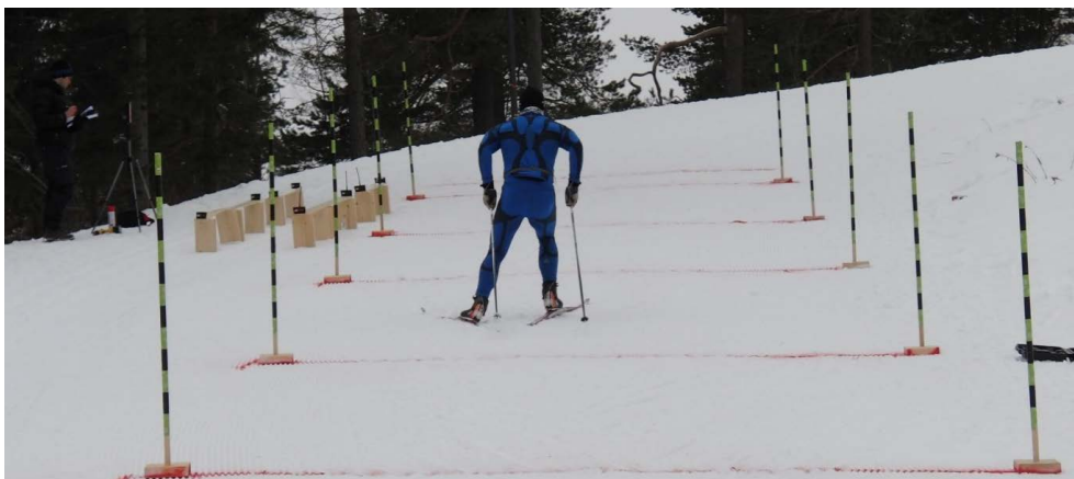
Figure 3.1. The 30 m-long outdoor data-collection area. To the left, photocells at fixed distances for calculating gliding friction.
