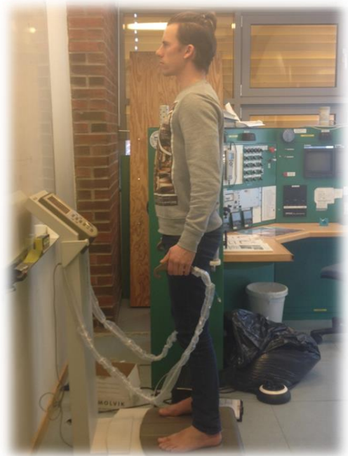
Figure 6: Image of subject standing with both feet on two electrodes while holding two electrodes in each palm measuring body composition with the Inbody 720
