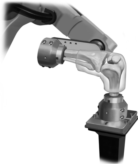
Figure 1. Schematic representation of the robotic setup with the inverted knee mounted in the testing system.
