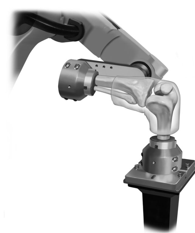
Figure 8. Schematic representation of the robotic setup with the inverted knee mounted in the robotic testing system.
