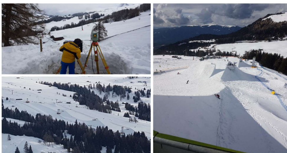
Figure 1. Pictures from the data collection in Seiser Alm. The upper left photo shows the tachy-meter based camera system, while the other two show the consecutive jumps.
