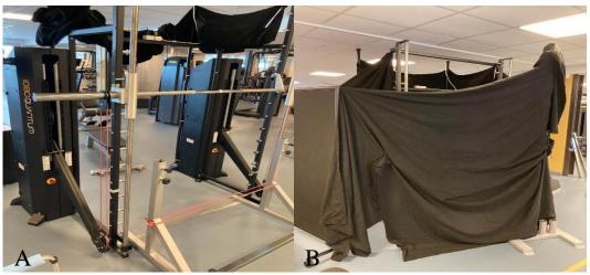
*Note*. 1080 Quantum system (1080Q) and Smith machine setup used in the experiment (A). Opaque cover around the 1080Q during testing (B).
