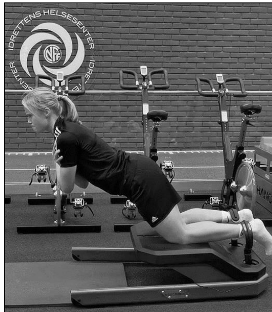
Figure 7. Picture of NordBord testing. The ankle braces are attached to load cells measuring the force when the player perform the Nordic hamstring exercise.
