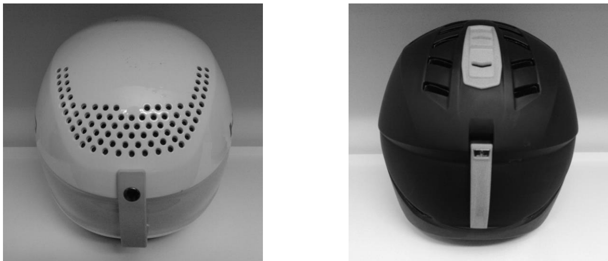
Figure 2. Rear views of the ski racing helmet (left) and recreational alpine sports helmet (right). Note that the recreational alpine sports helmet, both with and without RDS, had the same shell design.
